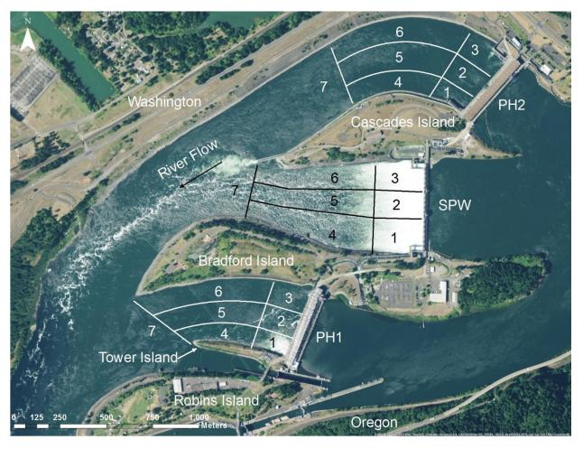
Figure 1. Bonneville Dam study area with Powerhouse One (PH1), Spillway (SPW), and Powerhouse Two (PH2) tailrace subareas separated into zones for assigning the location of predation events.
